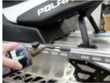
LEFT: The pictures here show installation prep tips to ensure proper adhesion. On metal surfaces, a butane torch can be helpful to clean and burn off oils.
