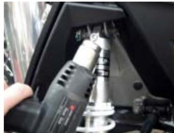
On plastic and painted surfaces, a heat gun is ideal to clean and warm surface. Warming the LED strip will make it more pliable and easier to bend.
