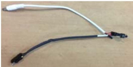
Wiring harness (white cable is input wire)
